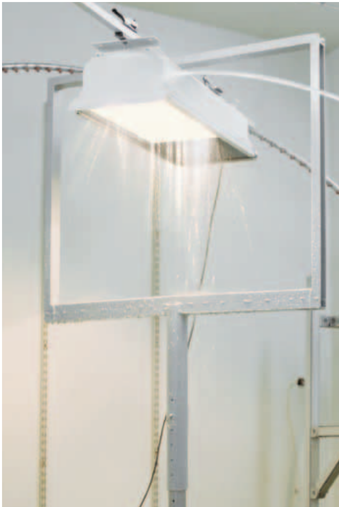
Water ingress protection testing
